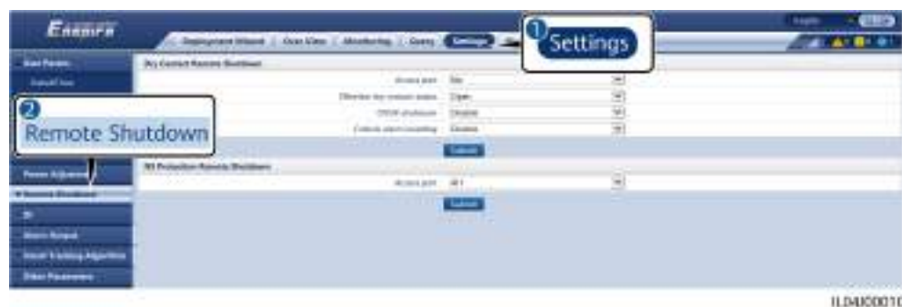
Figure 6-63 Dry contact remote shutdown
