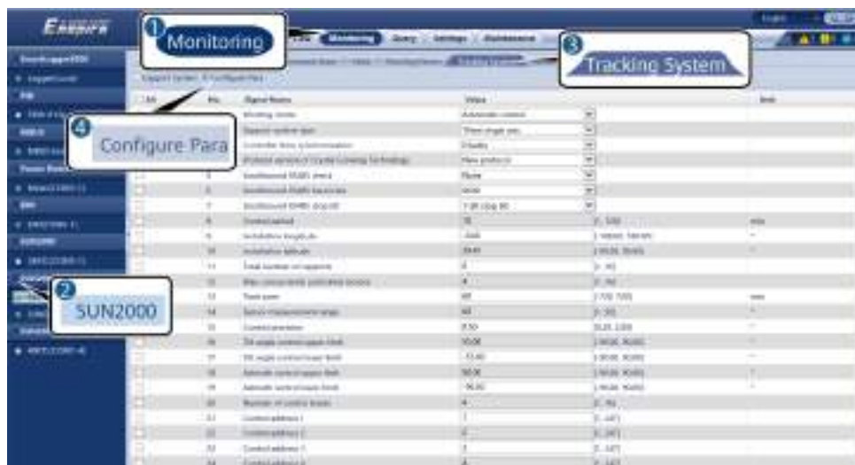
Figure 6-23 Setting configuration parameters (tracking system)
