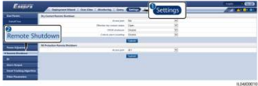
Figure 6-65 NS protection remote shutdown
